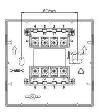
I1, I2: Zone in, connects to safe side of safety barrier or previous device, polarized
